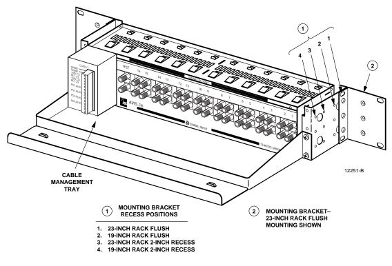
Figure 12. PWR-AVIS Chassis with Mounting Positions
